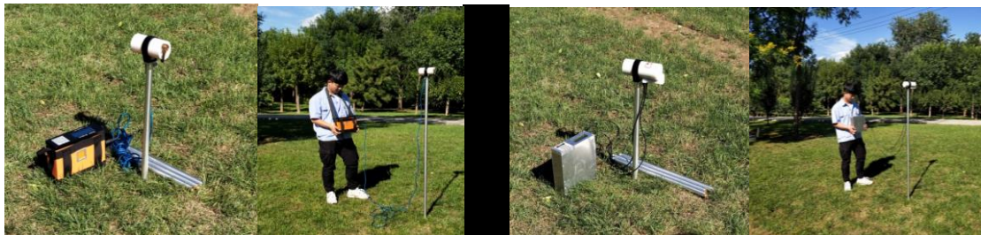
高精度直流激发型质子磁力仪 High precision direct current excitation proton magnetometer
