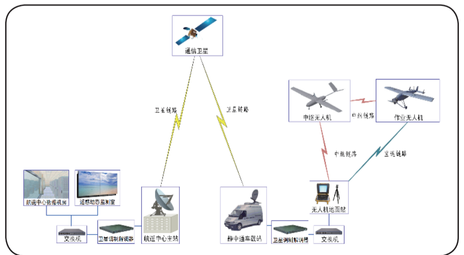
车载卫星通信系统拓扑图 Topological diagram of the satellite communication vehicle
